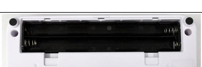
A photograph showing the black battery holder inserted into the battery compartment. The holder is now seated in the compartment.                                                                                      |
