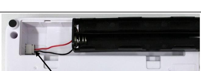
A photograph showing a black battery holder being connected to the metal contact point on the left side of the battery compartment. Red and black wires are visible, and a black arrow points to the connection point. |
